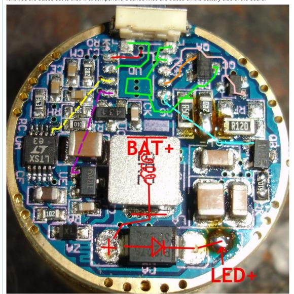
Pin #1 goes to B+. Pin #3 goes to the LTSX e3 boost controller, but it is NOT, from anything I am able to measure, a PWM-ed signal.
